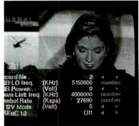
*On-screen set-up lets you see the data you're entering with the remote control. All the necessary numbers can be found at [www.lyngsat.com](http://www.lyngsat.com). Here are the parameters for receiving Deutsche Welle TV and Radio.*
