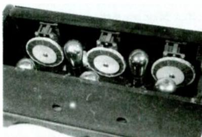
**FIG. 4.** A peek inside the set of Fig. 3 shows the set of five 01-A tubes and the three tuned circuits.
