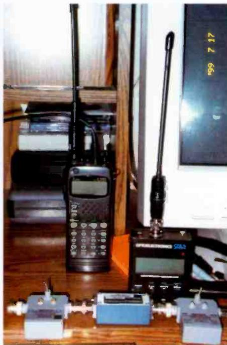
The Icom 32A shown with its computer interface cable plugged into the speaker jack. Alongside are my trusty Optoelectronics Scout and its FM and VHF paging filters.
