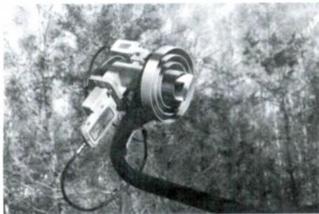
*Modified Teflon insert in throat of a C/Ku-band feed horn is the cheapest way to receive circularly polarized C-band signals and doesn't degrade linear C or Ku-band reception. (Courtesy author)*
