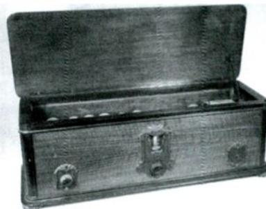
**FIG. 3.** RCA Radiola 60, an a.c. superheterodyne of 1928, used a retro cabinet design.
