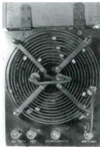
*BC-15A, Airplane Radio Telegraph Transmitting Set Box, looking at top of unit.*
