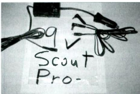
Author uses a 'Y' connector for two Pro scanners and Optoelectronics Scout. All take 9 volts.
