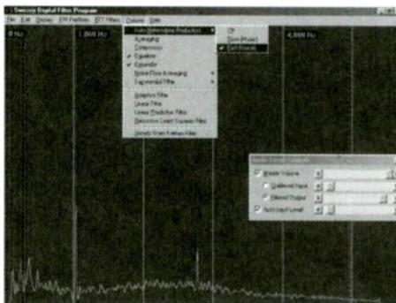
Figure 2 Swezey DSP in Automatic Heterodyne Rejection Mode
