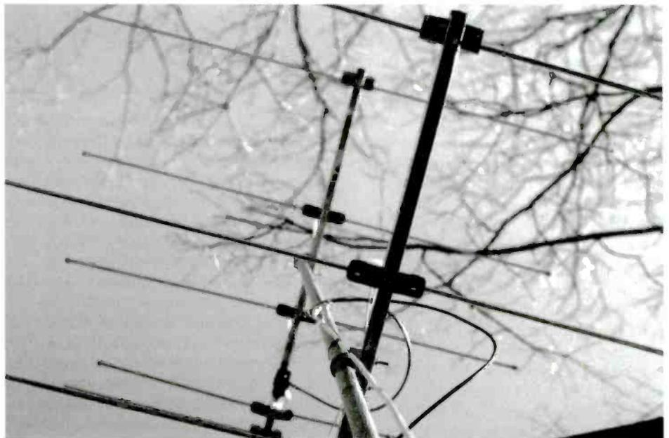
*Looking up at the stacked Yagis notice that all elements and the booms are parallel, mounted on the same side of the mast and facing the same direction!*
