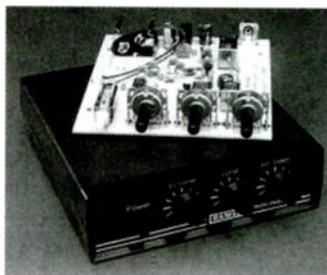
The SR-1 is a very sensitive (about a microvolt!) receiver. The superheterodyne design includes automatic gain control (AGC), radio frequency gain control, and plenty of speaker volume using any speaker or earphone. Smooth varactor diode tuning allows you to tune any 2 MHz portion of the 4 to 11 MHz frequency range. The kit runs on a 9 volt battery (not included). A matching custom case and knob set are available to give your radio a finished look.
