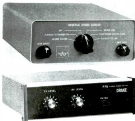
The patch connects to the telephone line. It also connects between a receiver and an external speaker. Phone patches for ham use provide transmitter connections, too, but you can ignore them for scanner applications.
