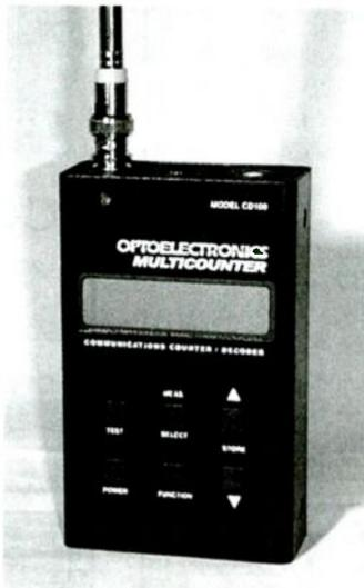
Optoelectronics has come out with the new Multicounter CD100 Counter/Decoder. The Multicounter combines a frequency counter and tone decoder in one handheld package. A great tool for the two-way radio technician, who can quickly check a whole fleet of portables for frequency and tone, the Multicounter is so easy to operate that even non-technical staff will find operation intuitive.
