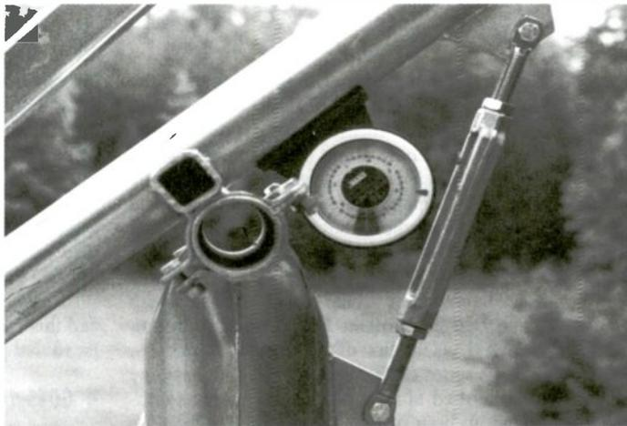
*Inclinometer in action. Helps check angles of your dish at the mount, on the pole and on the feed horn. Peaking the dish for optimum performance is easy and can save a service call. (Courtesy Ken Reitz)*
