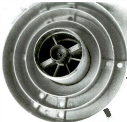
*Inside the feed horn cover of a C/Ku-band feed horn. Plenty of places for wasps to build their nests which could affect reception. (Courtesy Ken Reitz)*
