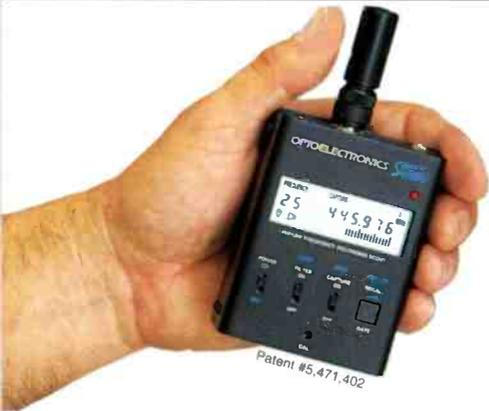
Capture the excitement of finding frequencies you never knew existed. The Scout locks onto the strongest signal in the nearfield and, in less than one second, displays the frequency.
