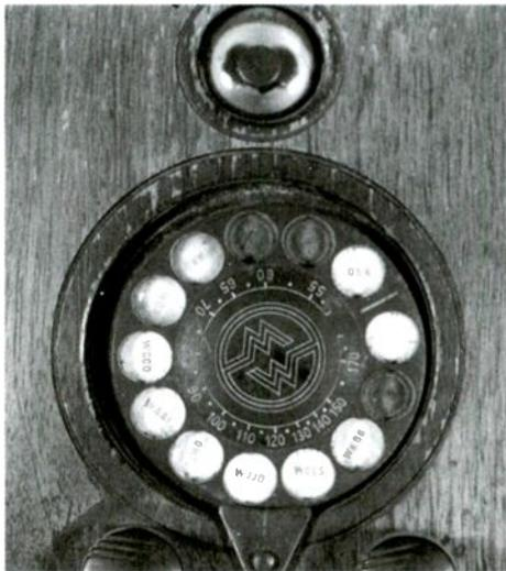
*1940s vintage Airline is equipped with both telephone-dial tuning and a tuning eye. This model is a vibrator-powered farm radio.*
