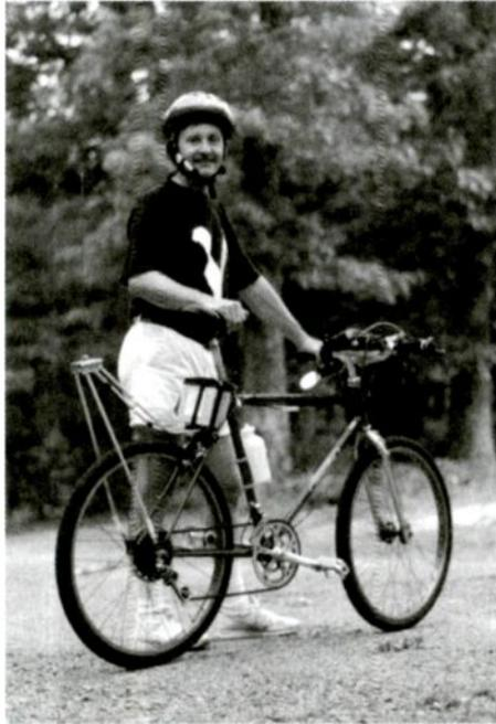
*1994 I'm racking up the miles going bicycle mobile, 21 gears no waiting! Note homebrew antenna support structure on back, motorcycle battery power supply under the seat, Alinco 2 meter mobile rig (up to 50 watts out!) and homebrew helmet mounted mike with push-to-talk mounted on the handle bars.*
