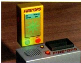
The system uses a personal unit to continuously monitor and record the fire-fighter's location and movement within a burning structure. Should the fire-fighter get lost, this unit will instruct the fire-fighter how to retrace his path of entry while also transmitting data that alerts a base unit located outside the structure.
