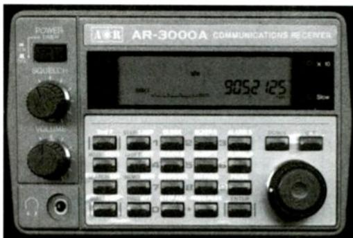
An internal lithium battery allows the digital clock to remember the time when power is interrupted. One can set the AR-3000A to turn on at a given time or turn off after a "sleep" interval, but we didn't use this feature.
