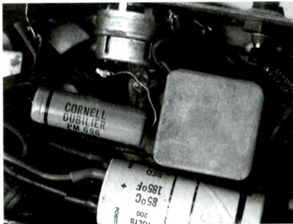
*Function of square-topped shallow metal can located under the chassis was a mystery until I checked the schematic. It turned out to be the second i.f. transformer.*
