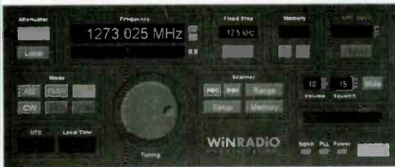
New WR-1550, with improved dynamic range! Continuous 150 kHz - 1500 MHz frequency coverage (less cellular), multimode detection (AM, NFM, WFM, USB, LSB, CW), IF shift (+/-2 kHz), sharp selectivity (2.5, 6, 17, 230 kHz), high sensitivity (0.3 uV SSB and NFM), built-in spectrum display, and triple superheterodyne conversion. This is the receiver that sets the standards!
