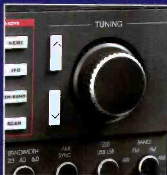
Ultra fine-tuning of 50Hz on LSB/USB, 100Hz in SW, AM and Aircraft Band and 20 KHz in FM.
