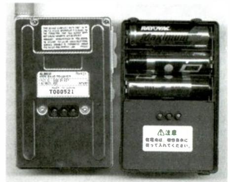
Figure 3. Rear view of DX-X2T (left) and the snap on, auxiliary battery pack/charger (right).
