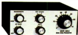
front panel output control; LO available via rear-panel jack for use with external frequency counter or digital dial; variable receiver offset tuning; four pole crystal IF filter with adjustable IF bandwidth
