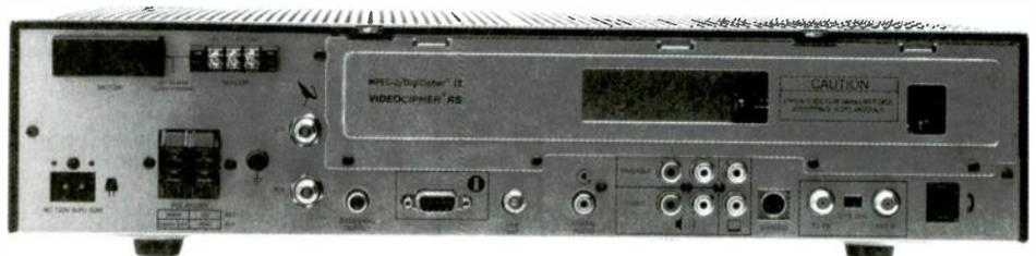
Rear panel of 4DTV features C/Ku-band LNB inputs, S-video output, fixed and variable audio outputs, external antenna input (for terrestrial TV), baseband video output (for stand-alone decoders), and slot for VCII decoder module. (Courtesy Motorola)
