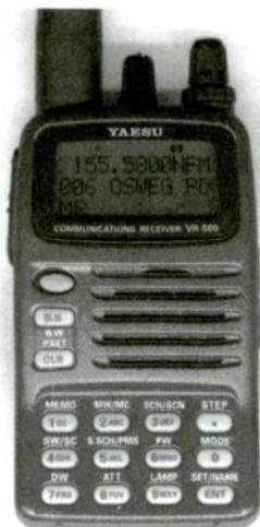
Figure 1. Yaesu VR-500 wide coverage receiver
