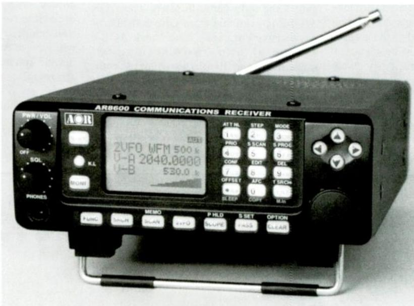
Front panel controls include volume (with on/off switch), squelch, and tuning. The LCD and all function keys are brilliantly lit (defeatable for battery conservation); signal strengths are displayed on a horizontal bar graph.
