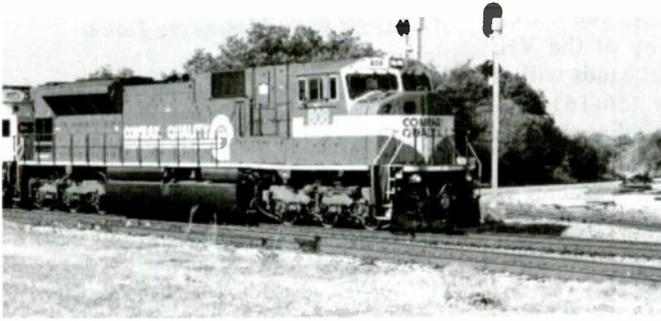
*Now owned by CSX, this former Conrail model SD8MAC locomotive generates 5000 HP and is equipped with DP, allowing it to be remotely controlled.*
