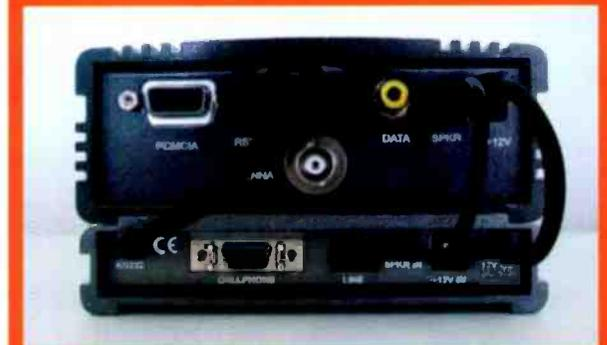
*WTCI mounted under a WR-3150e receiver (rear view).*
