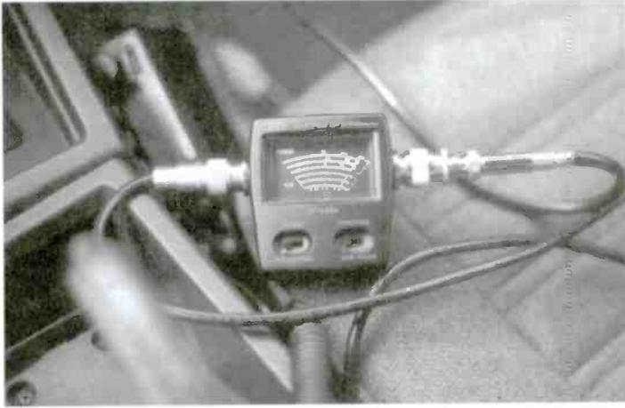
The MFJ-844 SWR/Power meter can be used to check the SWR and the power output of your HT or mobile transceiver. Here, the mini antenna checks out at 1.2:1
