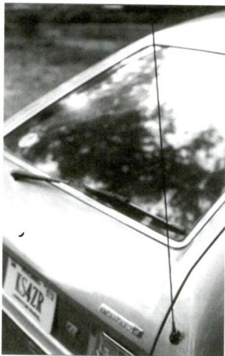
*Take a deep breath and go ahead and drill a hole in your car. This mini FM car antenna from Radio Shack adapts to just about any slope.*
