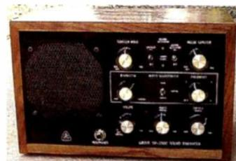
The Grove SP-200C offers variable-bandpass notch/peak function, separate bass and treble equalization, adjustable-threshold pulse-noise clipping, selectable-hold-time recorder activation, audio level, variable-hang noise squelch, and amplification. Processed sound is available through the high quality internal speaker, or from a headphone jack for secure installations or concentrated monitoring in noisy environments.
