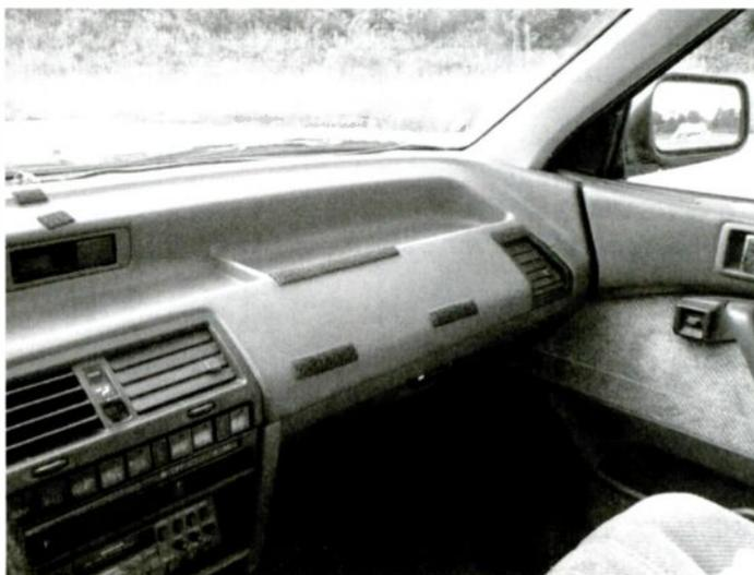
*A "before" photo of the empty dashboard, showing the Velcro strips used to mount the SWL portable radio*
