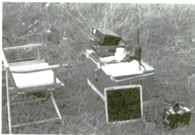
*Field Day 2001 gave me an opportunity to try out some minimal station ideas. The entire station including transceiver, transmatch, battery, solar panel, associated cables, wire and microphone fit nicely into the cooler with room for lunch. (Courtesy Author)*
