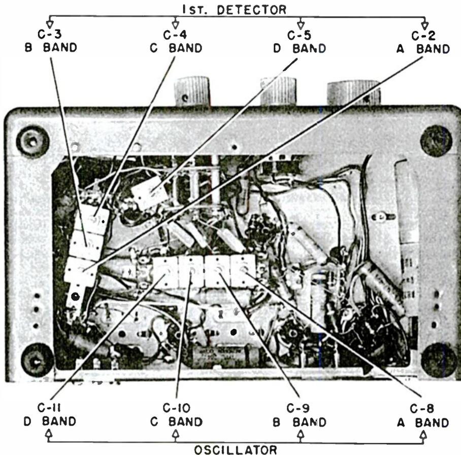
Illustration from instruction manual shows the oscillator and first-detector trimmers for the radio's four bands.
