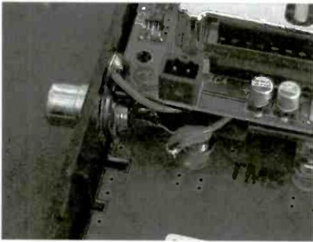
It is a tight fit, but it works great. For base scanners, there should be plenty of room on most models to drill a hole in the back of the case. Be sure to get all the metal shavings out of the inside of the scanner if you drill it. Note the location of the extra baseband audio RCA phono
