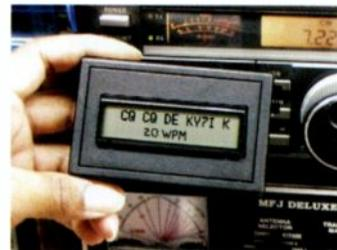
Better yet, if you need to store the decoded text, a serial port lets you display CW text on a monitor using a computer and terminal program. The MFJ-4612 can also be connected to your receiver with a cable, in case it's too noisy for microphone pickup or you don't want to listen to the signal. The pocket-sized reader operates on a 9-volt battery and defaults to sleep mode during periods of inactivity.
