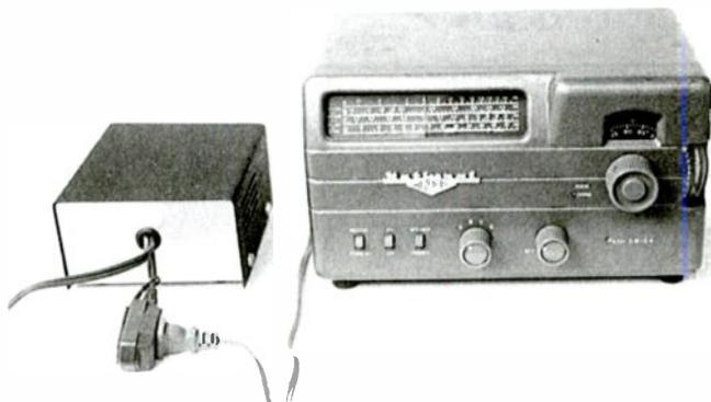
*The completed isolation transformer as set up to power the completed SW-54 for a final "smoke test" of both units.*
