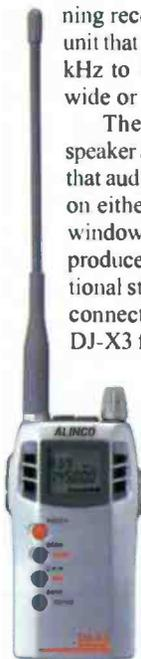
ning receiver, a pocket-sized unit that can receive from 100 kHz to 1.3 GHz in AM and wide or narrow FM modes.
