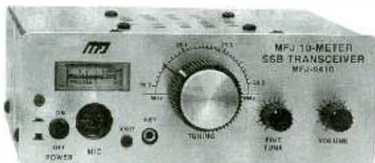
MFJ's 9410X is small, weighs only 2 pounds and puts out 20 watts (SSB) for fun HF mobile action (courtesy MFJ Enterprises)
