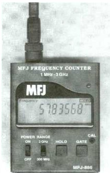
Figure 1: MFJ-886 frequency counter shown in Hold mode
