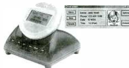
As you can see in the Figure, NetCallerID has a large LCD that displays caller ID information. The CD ROM supplied software is Windows 95 and 98 compatible and produces a pop-up window on your computer when you are connected to the Internet and an incoming phone call is detected. The pop-up window displays caller ID information and allows you to answer, log or ignore the call.
