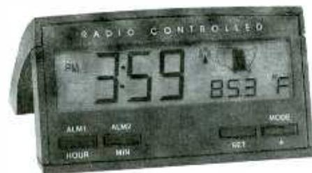
Radio-controlled clocks, such as this unit by La Crosse Technologies, take the guesswork out of timekeeping. Unit includes a built-in antenna for receiving WWVB's 60 kHz signal.
