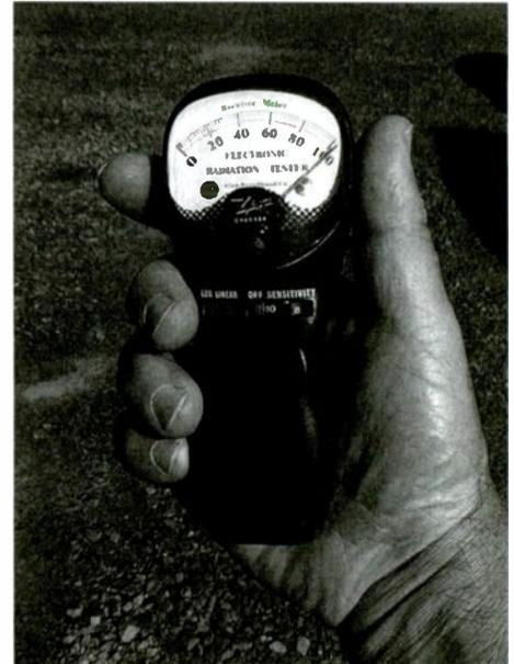
Designed to detect electromagnetic emanations from a large number of sources (microwave ovens, hidden transmitters, computer equipment, wireless phones, amateur and commercial two-way radios, etc.), the ZAP 180 boasts a wide frequency coverage of 10-4500 MHz (4.5 GHz).
