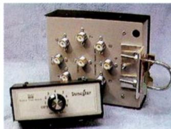
The Model 808 uses sealed 12vdc relays and a diode matrix select system to control the 8-positions on a 6-wire control cable. The relays operate reliably down to 9vdc. Unused antenna positions are grounded. The enclosure is all aluminum (black over gray) for maximum durability. Mounting is by a single U-bolt for simplicity and ease of installation. Connectors are UHF-type. Power handling 3kW. Requires 12VDC nominal at 200-ma maximum.
