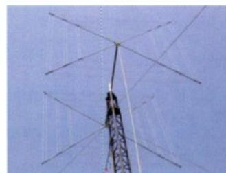
The antenna is called the "Baby Boomer Quad," also nicknamed "BBQ." The BBQ is a triband (10, 15 and 20 meters), reduced size, quad antenna with a single 50 ohm coax feed point; it does not require an antenna tuner. Weighing less than 30 lb it is designed for rooftop mounting using light-duty rotors and can be assembled and erected by just one person. The BBQ can be taken apart and packed in a box measuring just 8 inches square and 8 feet long.
