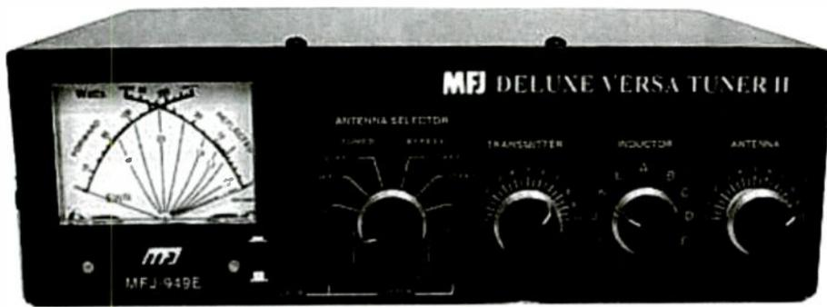
**MJF-949E Deluxe 300 Watt Tuner. Dubbed the Versa Tuner II, the 949E does multi-tasking in your listening post as an antenna coupler for three antennas, dummy load, transmatch, and SWR bridge. (Courtesy MFJ Enterprises)**
