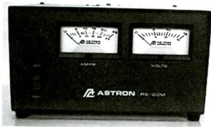
Astron RS-20M Power Supply. This versatile power supply gives you 13 volts at 20 amps and lets you read the voltage and current just to be sure. (Courtesy Astron Corp.)
