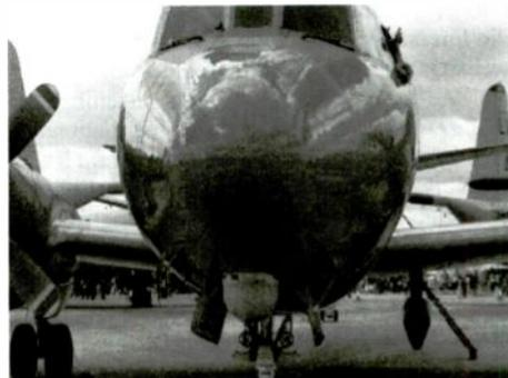
*This study of a Royal New Zealand Air force P-3 clearly shows the position of the nose camera. This is an early version of the P-3 with fixed turret. In US Navy variants, the turret retracts into the fuselage and is hidden from view.*
