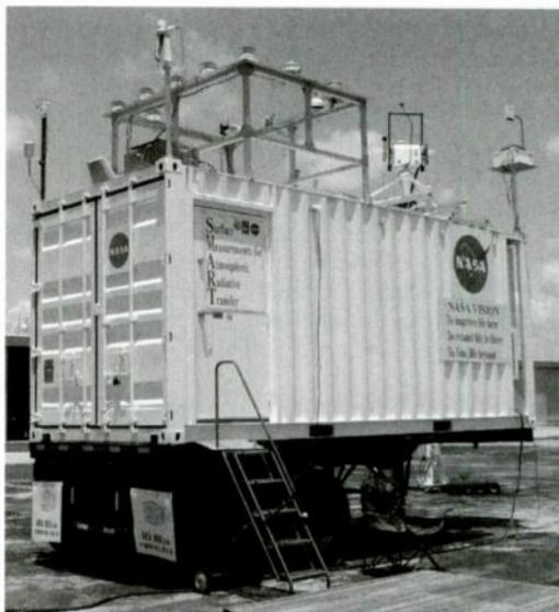
*Like a little science with your radio? NASA's Surface Measurements for Atmospheric Radiative Transfer (SMART) unit houses RF, Lidar and direct optical sensors for measuring cloud properties.*
