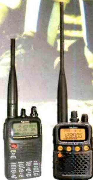
**VR-500 Carry the world with you.** (left) Providing continuous coverage from 100kHz–1299.99MHz (cell blocked), the 500 includes reception of narrow and wide-band FM, SSB, CW and AM. Featuring auto mode and frequency step selection, it aligns the user with standard configurations in use worldwide. It also sweeps a band, noting activity, quickly moving to active channels. 2.3" w x 3.7" h x 0.9" d, 7 oz ..... © **\$219.99**
