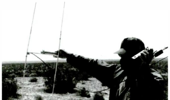
*A researcher uses a Sony multimode receiver and attenuator to track pulsed signals from tags on desert tortoises in California.*
