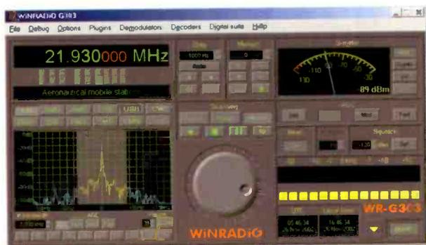
The G303i control panel includes many exciting features such as numerous tuning and scanning options, spectrum scope and others. (Professional Demodulator shown.)
