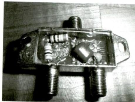
Fig. 4b: Diplexer with addition of 0.01 uF cap and split chokes
