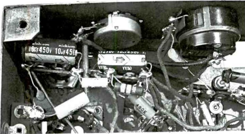
Newly-installed terminal strip (at upper left) holds the two replacement electrolytic caps and also provides a tie point to substitute for one that "disappeared" (see text). Volume and tone controls are at top of picture.
