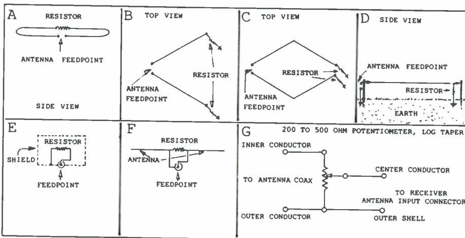
Fig. 1. A T<sup>2</sup>FD (A), a terminated-V (B), a terminated rhombic (C), a terminated Beverage (D), a dummy load (E), a low-SWR producer (F), the schematic for a simple variable attenuator (G).
