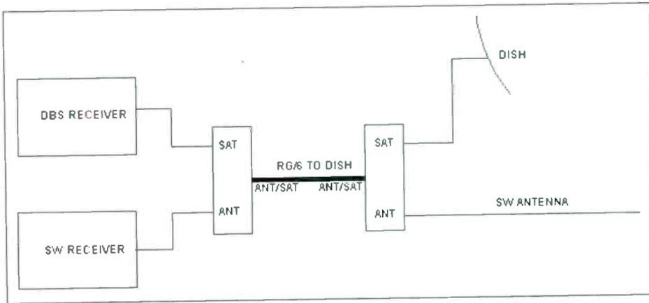
Fig. 5: Incorporating the diplexers into the satellite & SW antenna system.
