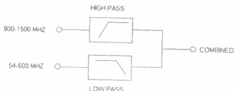
Fig. 1: Block diagram of a DBS diplexer
