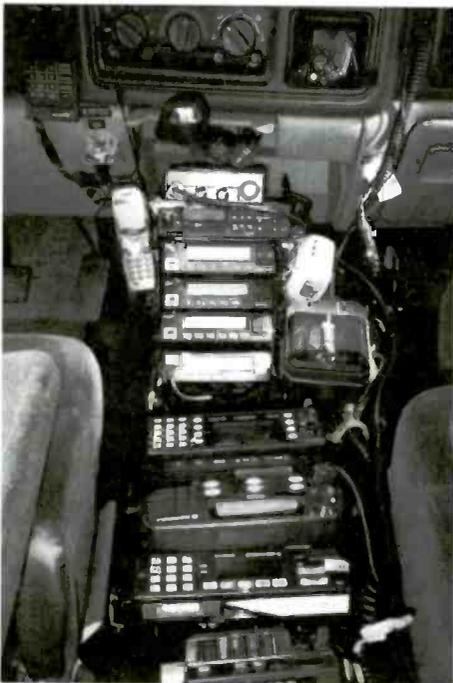
*My KPRC TV Rover truck setup. Radios are bolted down to deter theft. Radios with separate power units are kept in a locked cage. I keep radios that need the most adjusting at the top. J. Treadgold photo.*
