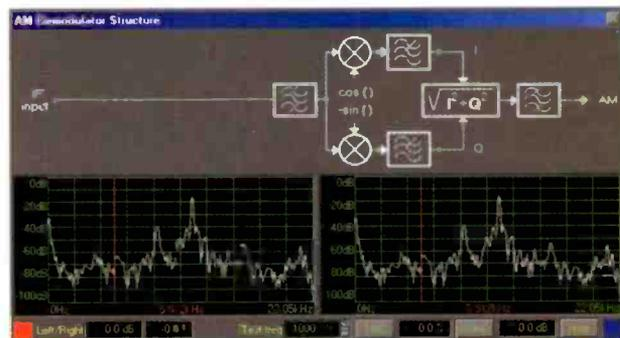
The Professional Demodulator contains an interactive block diagram for each modulation mode, two real-time spectrum displays and test facilities. A great tool to get familiar with *software radio* concepts.
