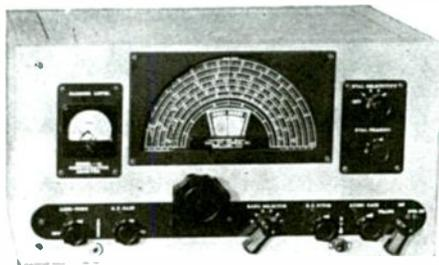
**Circuitry:** Transformer-powered superhet. One r.f. stage; two i.f. stages; bandspread; "s" meter; crystal filter; BFO; noise-limiter;
