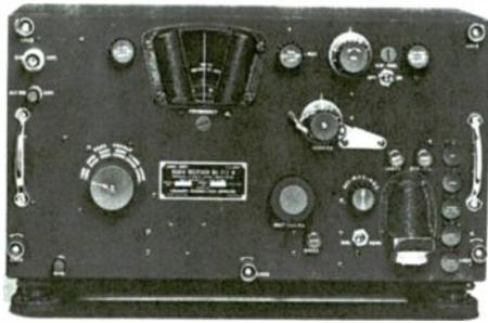
**Circuitry:** Dynamotor-powered (BC-312) or transformer-powered (BC-342) superhet. Two r.f. stages; two i.f. stages; crystal filter (some models); BFO; speaker separate. *Tube complement:* 6K7 (2) 1st and 2nd r.f. amplifiers; 6L7 mixer; 6C5 oscillator; 6K7 (2) 1st and 2nd i.f. amplifiers; 6C5 BFO; 6R7 detector/1st audio; 6F6 (audio output).
