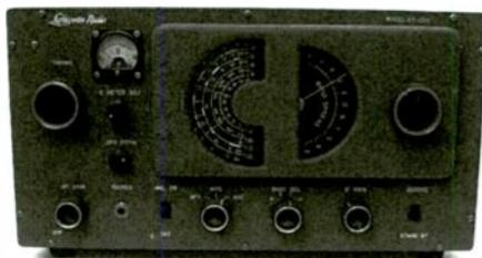
**Circuitry:** Transformer-powered superhet. One r.f. stage; two i.f. stages; bandspread; S-meter; BFO; noise-limiter; speaker separate. *Tube complement:* 6BD6 r.f. amplifier; 6BE6 oscillator/mixer; 6BD6 (2) 1st and 2nd i.f. amplifiers; 6AV6 detector/AVC/1st audio; 6AV6 BFO/limiter; 6AR5 audio output; 5Y3 rectifier.
