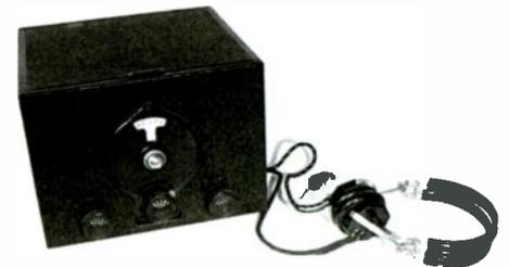
**Circuitry:** One r.f. stage; regenerative detector; one stage of audio; headphone operation only. *Original Tube complement:* **for battery operation** 36 r.f. amplifier; 36 detector; 37 audio output **for a.c. or a.c./battery operation** 35 r.f. amplifier; 35 detector; 27 audio output.
