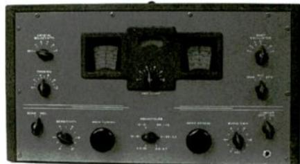
**Circuitry:** Transformer-powered superhet. One r.f. stage; three i.f. stages; voltage-regulated oscillator; bandspread; "s"-meter; crystal filter; BFO; noise-limiter; speaker separate. *Tube complement:* 6SS7 r.f. amplifier; 6K8 oscillator/mixer; 6SS7 (3) 1st, 2nd and 3rd i.f. amplifiers; 6H6 detector/noise limiter; 6SN7 1st audio/S-meter amplifier; 6SJ7
