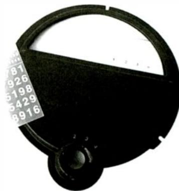
*A computer-generated number strip was created as a template for replacing wiped-off numbers on the dial window (see text) with properly-sized dry-transfer numbers selected from a hobby-shop sheet (corner seen at left).*
