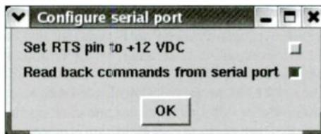
There are several different PC cloning cables from which to choose and tk5 and tk10 let you alter two serial port settings to function with various cables. Experimentation is required to find the correct settings for your cable.
