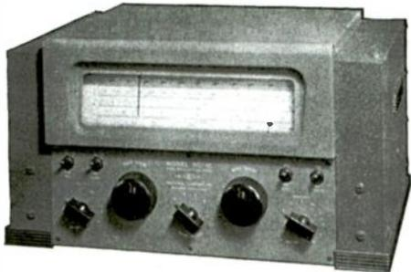
**Circuitry:** A.c.-d.c. superhet (no power transformer). No r.f. stage; two i.f. stages; push-pull audio output; bandspread; BFO; noise limiter; speaker separate. *Tube complement:* 6K8 oscillator/mixer; 6SG7 (2) 1st and 2nd i.f. amplifiers; 6H6 detector/limiter; 6SF7 AVC amplifier; 6SJ7 BFO; 6SC7 phase inverter; 25L6 (2) audio output; 25Z5 rectifier.
