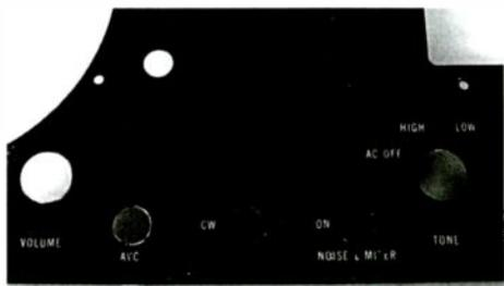
*Close-up of cleaned-up panel shows my unfortunately-necessary patch on the paint surrounding the AVC switch location. Silk-screened "noise limiter" label was already damaged.*
