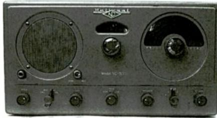
**Circuitry:** Transformer-powered superhet. One r.f. stage; two i.f. stages; voltage-regulated oscillator; bandspread; BFO; noise-limiter; built-in speaker. *Tube complement:* 6SG7 r.f. amplifier; 6SBY7 oscillator/mixer; 6SG7 (2) 1st and 2nd i.f. amplifiers; 6H6 detector/AVC/limiter; 6SN7 1st audio/BFO; 6V6 audio output; VR150 voltage regulator; 5Y3 rectifier.
