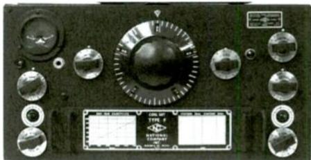
**Circuitry:** Features and tube lineup varied over the years. Model illustrated has two r.f. stages; two i.f. stages; separate mixer and local oscillator; crystal filter; combined detector and AVC stage; first audio amplifier; noise limiter; audio output stage; CW oscillator; "S" meter. Requires separate power supply and speaker.
