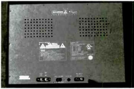
Rear panel features genuine Masonite back complete with unnecessary air-holes. Antenna terminals (left) allow serious antenna connection while antenna jack (right) is for the AN-03 roll-up antenna which is included with the radio. RCA stereo input jacks allow hook-up for CD, cassette or other accessory. (Courtesy: Author)
