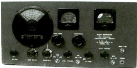
**Circuitry:** Transformer-powered superhet. Two r.f. stages; two i.f. stages; push-pull audio output; bandspread; "s" meter; crystal filter; BFO; noise-limiter; speaker separate. *Tube complement:* 6SK7 (2) 1st and 2nd r.f. amplifiers; 6K8 oscillator/mixer; 6SK7 (2) 1st and 2nd i.f. amplifier; 6SQ7 detector/AVC/1st audio; 6H6 noise limiter; 6SQ7 phase inverter; 6J5 BFO; 6F6 (2) audio output; 80 rectifier.
