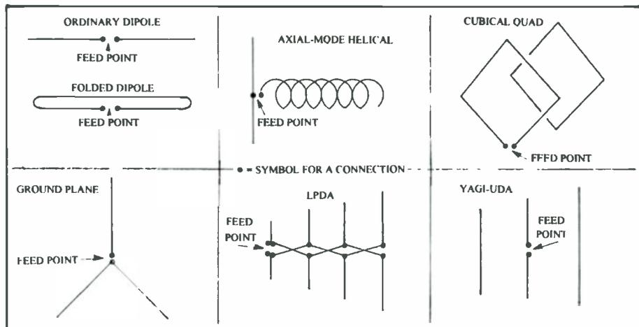
Fig. 1. Circuit diagrams for some common antenna types.
