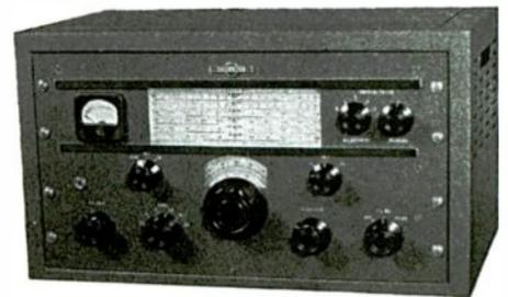
**Circuitry:** Transformer-powered superhet, ham bands only. Double conversion. One r.f. stage; two mixers; three i.f. stages; bandspread; "S" meter; crystal filter; BFO; noise-limiter; speaker separate. *Tube complement:* 6AK5 r.f. amplifier; 6SA7 1st mixer; 6SK7 1st i.f. amplifier; 6L7 2nd mixer; 6AK5 crystal oscillator; 6SG7 (2) 2nd and 3rd i.f. amplifiers; 6H6 detector/limiter; 6SJ7 BFO; 6SJ7 1st audio; 6V6 audio output; 6SJ7 VFO, 5Y3 rectifier.
