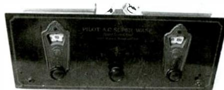
**Circuitry:** One r.f. stage; regenerative detector; two stages of audio; separate speaker (not supplied). *Tube Complement:* **battery version** 22 r.f. amplifier; 01-A detector; 01-A first audio; 01-A audio output **a.c. version** 24 r.f. amplifier; 27 detector; 27 first audio; 27 audio output.
