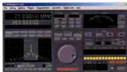
The optional Professional Demodulator expands the receiver capabilities yet further, by introducing additional innovative features: continuous selectivity setting (1 Hz to 15 kHz in 1 Hz increments), interactive demodulator diagrams with real-time audio spectrum scopes and vector voltmeters, built-in performance test facilities (it even lets you measure the receiver's own sensitivity), and many others.
