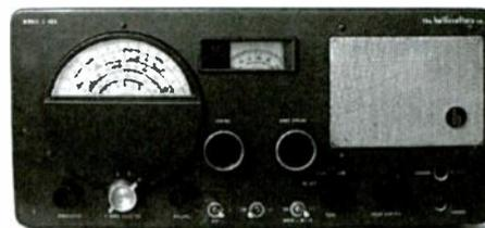
*S-40A with front panel reassembled. I think it looks quite sharp now, even though it's far from mint. Unoccupied holes at right are for standby/receive switch and phone jack (see text).*
