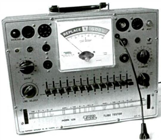
*Attractively-packaged Eico 628 emission tester has been on my bench for some time because it checks some of the last consumer types manufactured (which are not covered by my TV-7). It's handy for checking out the occasional TV set.*
