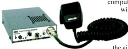
Best of all, the ARD9800 works with your existing transceiver. The ARD9800 requires only two connections to any ham radio, one through the radio's microphone input port, the other from the rig's "speaker out" jack to the ARD9800's audio input port. No modifications to the radio are necessary. You may use the microphone provided with the ARD9800 or wire your mic to work through the ARD9800.
