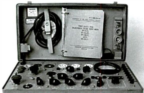
*The military TV-7 is my mainstay tube tester. It covers a very wide range of tubes from the 1920s through the 1960s, and even handles some low-and medium-powered transmitting types.*
