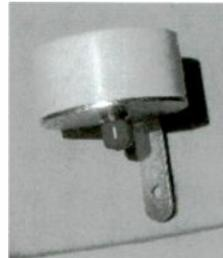
Next, we tried the "Ultra-M Beam," a 4-inch directional antenna with a claimed gain of 12 dBi (approximately 10 dBd). The AVCOM spectrum analyzer verified higher gain over the Omni – signal spikes were about 5 dB higher than seen for the Omni in our field experiments.
