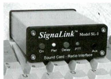
*This multi-mode interface lets you monitor all the action on 10 meters. You can view CW, RTTY, SSTV, Packet, and more on your computer screen. (Courtesy TigerTronics)*
