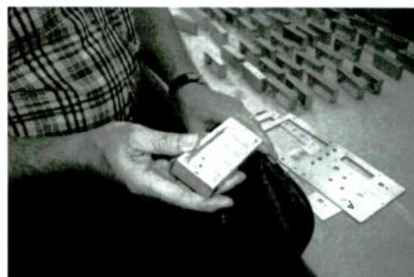
*Ken displays recently milled aluminum filter cavities*
