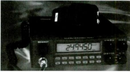
**Ranger 10 & 12 meter transceiver. A great entry level rig for getting started on 10 meters. It's small and relatively inexpensive making it a great base or mobile radio. (Courtesy Ranger Communications, Inc.)**
