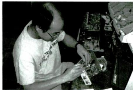
*Machine Shop Foreman Tinh Ha completes the final assembly of a Frequency Extender Unit*
