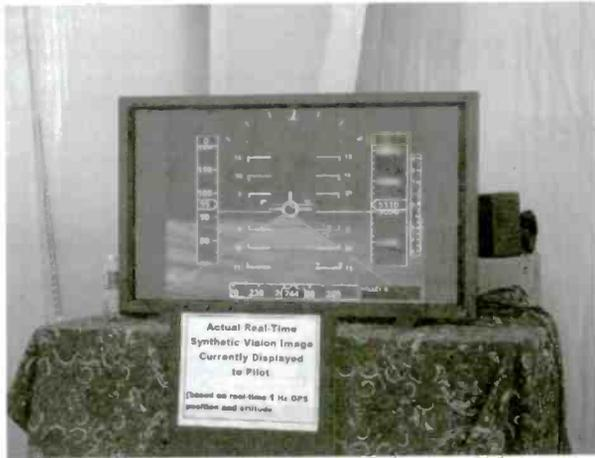
A large screen shows in real-time the display seen by the pilot as he follows the approach path (Rachel Baughn)
