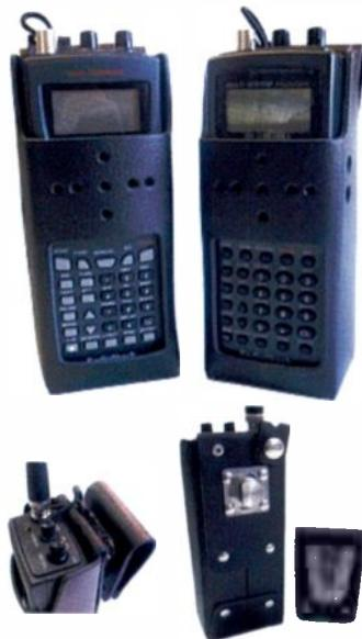
The Scanner Master PRO-92/95 case also includes a quick-release swivel unit. The swivel piece stays on your belt while you can turn the radio upside down and pull it, while in the case, off your belt. If the user is worried about the radio staying secure in the case, a quick-release bungee cord can be placed around the BNC jack at the antenna.
