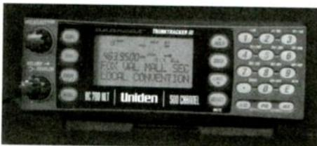
conventional memory channels. Wide frequency coverage, alpha labels, CTCSS and DCS squelch, tuning knob, computer control. The price of used BC780XLTs is starting to drop below the \$200 range.
