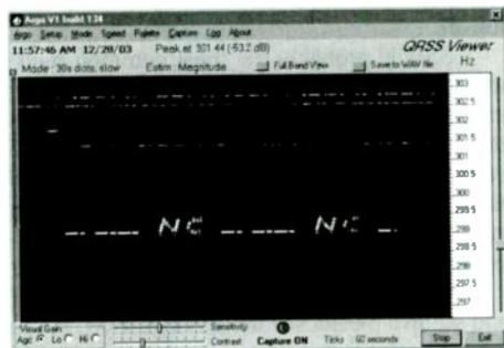
The website at [www.w3eee.com](http://www.w3eee.com) allows a near real-time glimpse into the world of QRSS. This image shows Lowfer "NC" displayed on the site.
