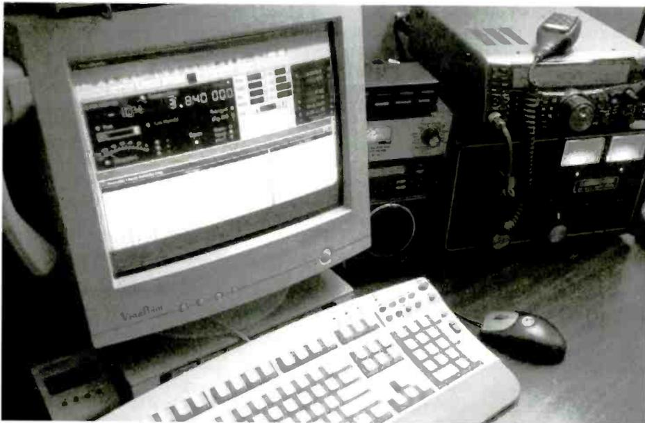
If you have modern ham equipment and antennas, you may be as close to setting up your own online tuner with just some additional software. Pictured here with the Kenwood TS-2000 which will work out of the box with VisualRadio. Many other modern transceivers will work as well.
