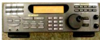
Some of the other published features include a RS-232 DB9 PC interface, display backlight, priority scan, trunk scan and search, one-touch weather reception, SAME weather alert, AutoStore and much more. The case style and basic operation of the BC-898T remain unchanged from the previous model.
