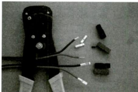
I then use a quality wire stripper to take off about 1/4 inch of the insulation. I give the bare wires a quick smooth right hand twist. I carefully insert the wire into the coupler with a right hand twist motion. I use the wire strippers as a holding vise and solder on the connectors. The red (positive) wire should be closest to you. Note how the connectors are "upside down" for the solder to flow properly.
