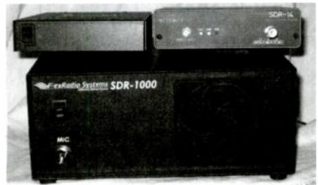
Figure 2 - FlexRadio SDR 1000 Transceiver with RFSpace SDR-14 and ICOM PCR1000 receivers sitting on top.
