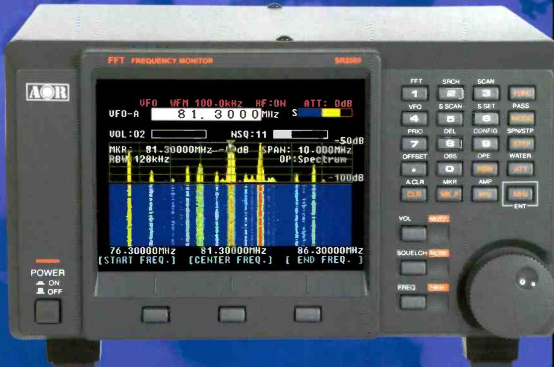
**The SR2000 is an ultra-fast spectrum display monitor with a high quality triple-conversion receiver**
