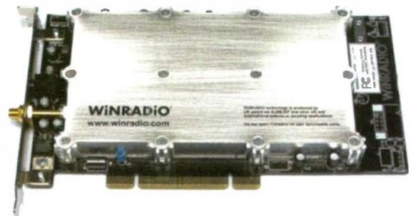
*WiNRADiO software-defined high-performance HF receiver (internal PCI card and external USB versions are available)*
