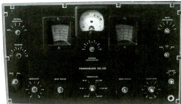
*The restored front panel now fitted to the chassis of the former parts set and ready for installation of the knobs.*
