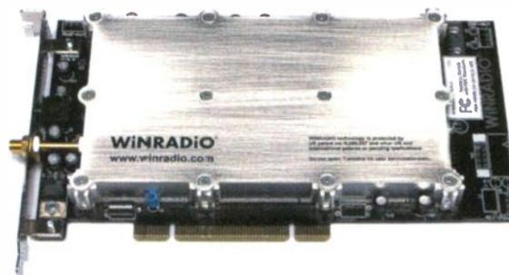
*WiNRADiO software-defined high-performance HF receiver (internal PCI card and external USB versions are available)*
