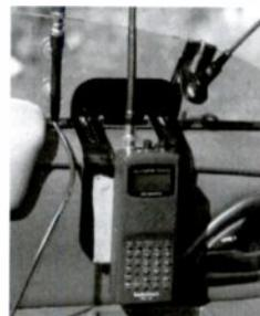
*Easy and cheap approach: HT scanner mounted on driver's window with a cheap metal bookend, shown with two types of optional window antennas for HTs.*
