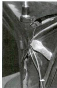
*Ham 2 meter hood antenna, and direct battery DC power cables running from engine compartment to the inside of driver's area, under the dash over to the DC power strip. The Antenex screw on antenna can be easily swapped out for other bands.*
