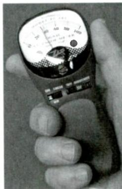
As expected, some environments are packed with radio-frequency (RF) signal sources, and the ZC185 is, after all, a field strength meter; as such, it provides a reading of the aggregate of all signals in the environment. Nonetheless, as discrete signal sources are approached, the readings get stronger.
