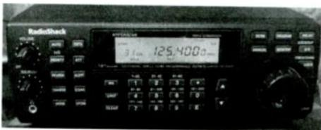
*This Radio Shack PRO-2045 (discontinued) is an example of a scanner with a tuning knob. One can manually tune up and down through frequencies, through a search range, and through programmed channels. It is a very handy but uncommon feature.*
