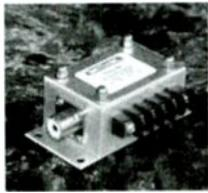
*Feed your Beverage! This 9:1 Balun is for Beverage antennas with 4 taps for different impedances. Transforms your Beverage antenna to match 50 ohm coax. (Courtesy: Industrial Communication Engineers)*
