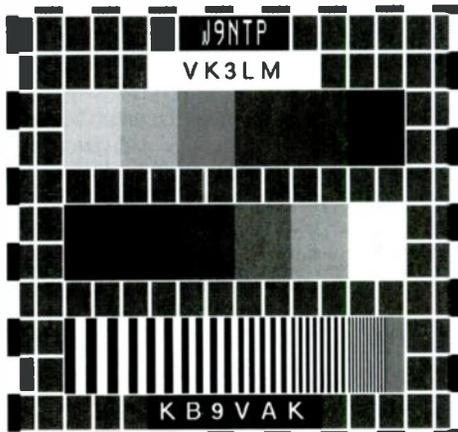
Transmission tests on 20 meters of HDSSTV (later renamed Redundant Digital File Transfer, RDFT-SSTV) between VK3LM (Australia) and W9NTP (U.S.). The first figure shows an analog Robot36 SSTV 30.5 second transmission. The second figure shows a 30.5 second RDFT-SSTV transmission. (Courtesy: Barry Sanderson, KB9VAK's web site: <http://www.svs.net/wyman/examples/hdsstv>)
