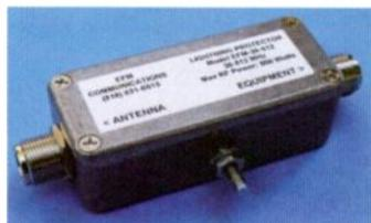
The EFM lightning protector presents a DC short between the center pin and shield on the antenna port, and a DC open between the center pins of the antenna and equipment ports. It is designed to be used in systems where there is no DC voltage on the coax to power tower-mounted electronics.
