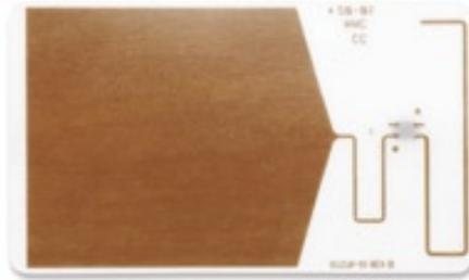
**Windshield mounted 915 MHz RFID tag from Intermec for toll and parking access.** (Courtesy: Intermec)
