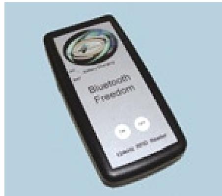
*TEK Industries Freedom HF Bluetooth hand-held RFID reader/writer works industry standard 13.56 MHz RFID tags. (Courtesy TEK Industries)*
