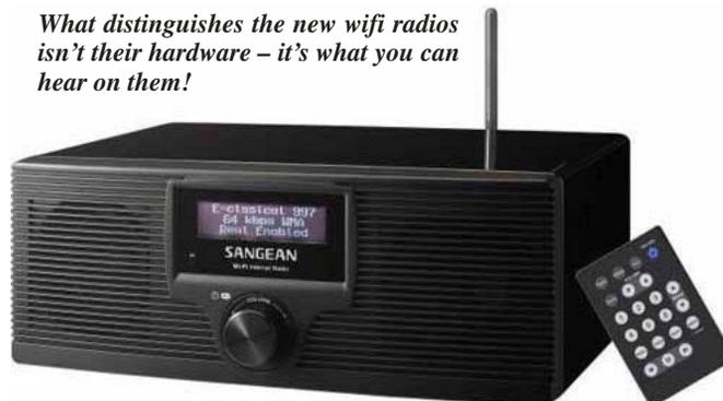
The WFR-20 is powered from AC; internal audio power to its speakers is 5 watts per channel, available for optional external speakers or a set of headphones from rear terminals. To feed the receiver's audio to an external amplified stereo system, a stereo line output is also provided. Both audio sources employ standard 3.5 mm (1/8") jacks.
