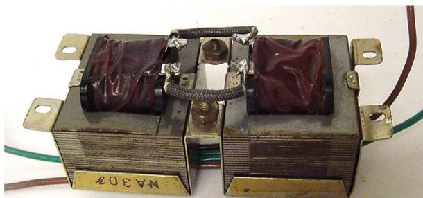
Fig. 1. Isolation transformer made from two low-voltage transformers with secondaries connected (see text).
