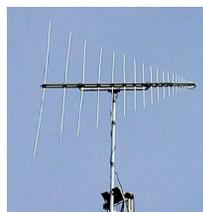
**VHF-UHF Log periodic dipole array (LPDA) receives 105-1,300 MHz (17 elements on a 4' boom): \$300.** (Courtesy: Create Antennas)
