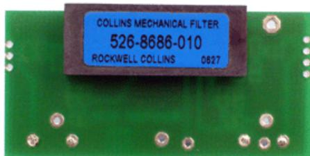
*W4RT add-on, inboard Collins Mechanical Filter for Icom 718 \$114 if you install it yourself. (Courtesy: www.w4rt.com)*
