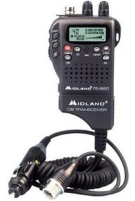
*Midland Radio 75-822 (\$125) is a microphone-sized, full-featured CB with NOAA weather radio, but it's useless without an external antenna. (Courtesy: Midland Radio)*
