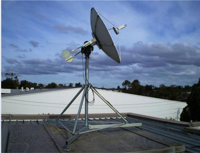
WiNRADiO has added a new product to its large range of innovative receivers and radio monitoring and surveillance systems: The WSS-420 turn-key weather satellite monitoring system.
