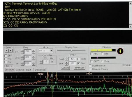
Typical RTTY screen shows the distinctive twin peaks of a RTTY signal, in this case, RK6CK, Temyruk, Russia. (Courtesy: Author)
