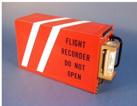
*An example of a Cockpit Voice Recorder (CVR). They record four channels of audio that includes radio transmissions, cockpit voices, and other sounds. Photo courtesy National Transportation Safety Board (NTSB)*
