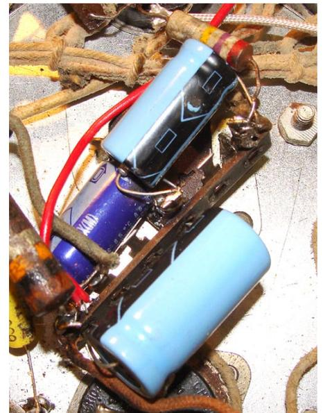
Three new electrolytic capacitors used to replace an original can type. Note arrows indicating negative terminal on top capacitor.
