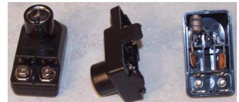
“They come with what’s called a Type F connector. It is a stud fitted into the plastic with a metal shell around it. These pieces can be removed – carefully – and a 3/8 inch hole drilled for a female BNC connector – also done carefully. If the drill goes too fast, the plastic will melt, the drill bit will stick, and the whole caboodle will turn into a bunch of little pieces.”
