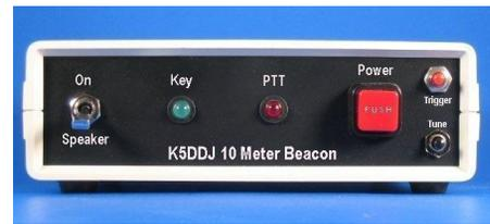
*A homebrew 1/2 watt beacon transmitter made from a 27 MHz pocket pager. After changing the crystals, retuning the pager, and repackaging the unit, K5DDJ made a really nice unit. It has been on the air 24/7 since 2006. (Courtesy K5DDJ.com)*
