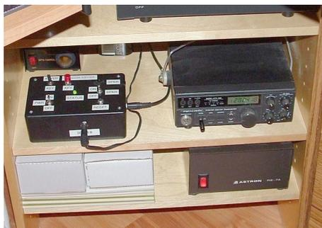
*The 10 meter Beacon stowed under my primary operating desk. The keyer is in the black box to the left. The small power supply on the lower shelf powers the HTX-100. The large power supply on the top shelf powers the main equipment in the station. (Courtesy: Author)*
