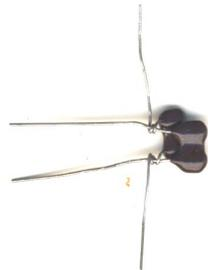
Figure 2: Capacitors in Parallel
