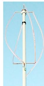
*The Quadrifilar Helix antenna is a relatively easy to build, omnidirectional antenna that can be optimized for both amateur radio and weather satellite work. (Courtesy: Bob Cash, N8IMO)*
