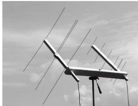
*Satellite antennas don't need to be fancy to be effective. Here, a pair of vertically polarized, "home brew" Yagi antennas made from bits of wire and wood are mounted on a wooden cross boom. (Courtesy: AMSAT)*
