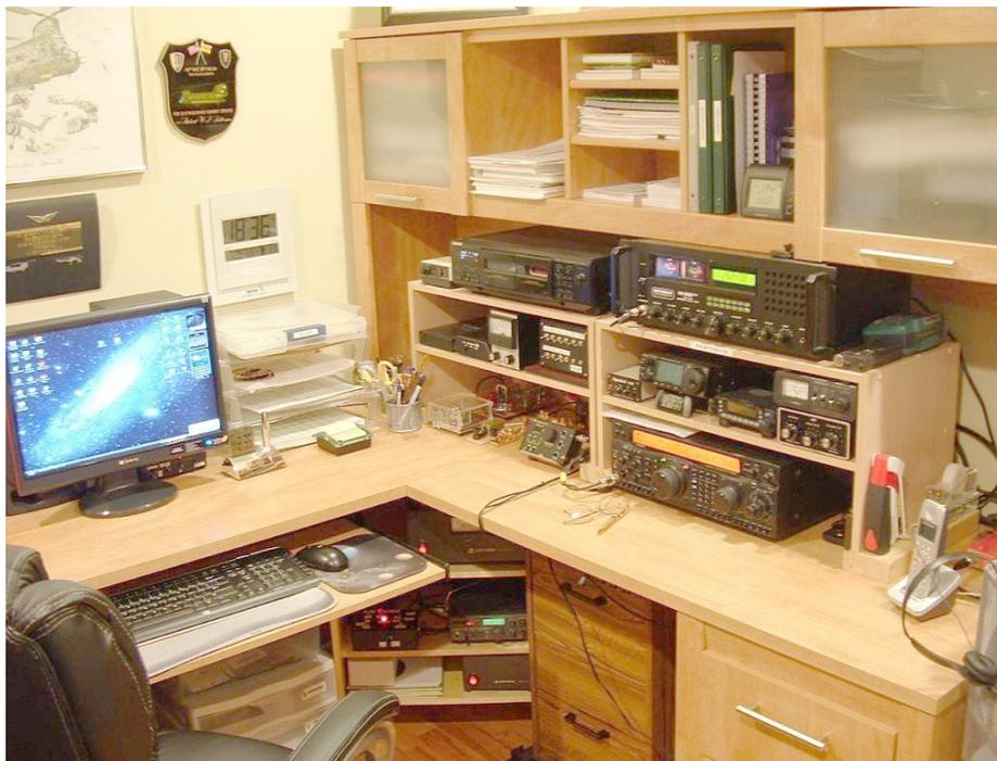
*The main operating position at K5DZE shows the 10 meter beacon under the desk in the lower center of the picture. It is well out of the way, but easy to access. (Courtesy: Author)*
