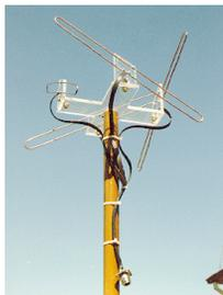
*The Lindenblad antenna is yet another, relatively easy to build omnidirectional antenna suitable for satellite work. (Courtesy: AMSAT)*
