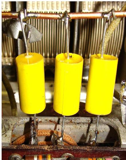
*Bottom leads of replacement r.f. tube shelf capacitors are soldered to cut-off terminals of original can capacitor sections.*
