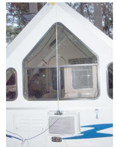
*A mobile HF whip is a simple solution to campsite antenna limitations*
