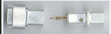
*This two-piece, Type-N connector makes the age-old chore of working with N connectors a breeze. (Courtesy: Universal Radio)*
