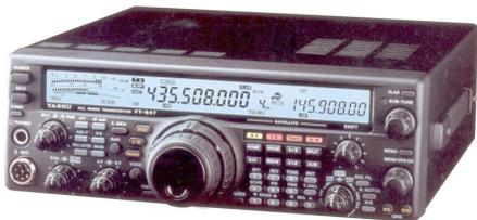
*The Yaesu FT-847 is a 1990s-era, all-mode, HF/VHF/UHF base station radio that was specifically optimized for full duplex satellite work. While now out of production, it can sometimes still be found on the used market. (Courtesy: www.rigpix.com)*
