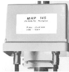
*Mast-mounted preamps, such as this one from SSB electronics, boost weak satellite downlink signals at the antenna feed point where those signals are strongest. (Courtesy: SSB Electronics)*
