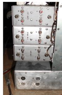
*The first r.f., second r.f. and first detector cans, with four trimmers each, are above. The four oscillator trimmer access openings, with covers in place, are below.*
