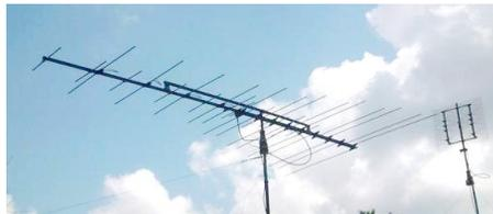
*Author's TVDX antennas: a Winegard VHF antenna (left) and a Channel Master 8-Bay UHF antenna (right). The UHF antenna is connected to a Winegard preamp. Both are on rotators. (Courtesy: Author)*
