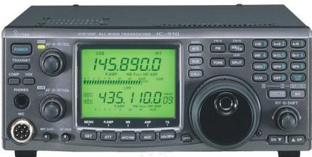
*The ICOM IC-910H is a late model, all mode VHF/UHF base station that was specifically optimized for full duplex satellite work. This radio has recently been dropped from the ICOM lineup in favor of a newer satellite-capable model. However, Start looking for the ‘910H to show up on the used market. (Courtesy: www.rigpix.com)*
