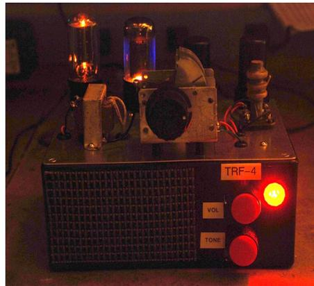
used to be hidden inside wooden or plastic cabinets behind fancy dial faces. This project would be different, highlighting the four constituent tubes.
