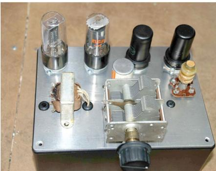
This is a standard tuned radio frequency (TRF) AM broadcast receiver that doubles as a small audio amplifier. After all, who can resist the soft glow and warm tones generated by receivers equipped with this technology? Tubes
