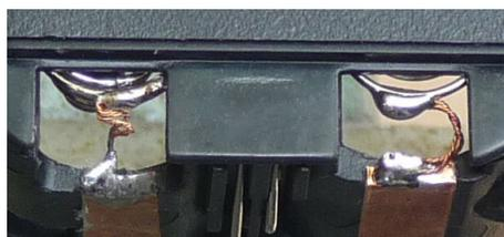
Figure 5. Battery contact to conductor connection
