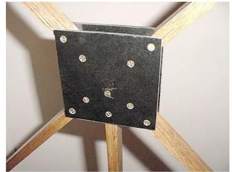
*Detail of the center of the loop showing the square pieces screwed to the arms and mast.*
