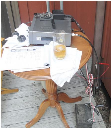
*KS4ZR Field Day 2010 operating position. As the ice quickly melts in the 90+ temperature I wondered, "Would 10 watts and a 20' section of rain gutter 10 feet off the ground be enough to be heard?" The iced tea really helped.*
