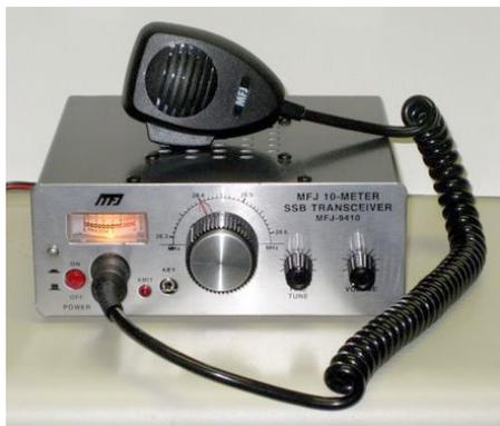
The control panel is simplicity itself. A tuning knob adjusts the frequency (28.3-28.6 MHz), and a volume control selects comfortable audio from the internal 3” speaker.
