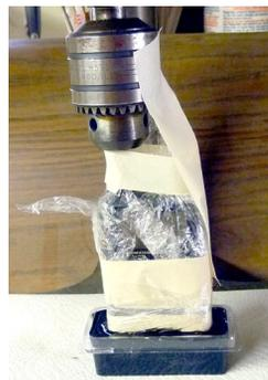
Figure 6. Wrapped VR-500 lowered into the epoxy.
