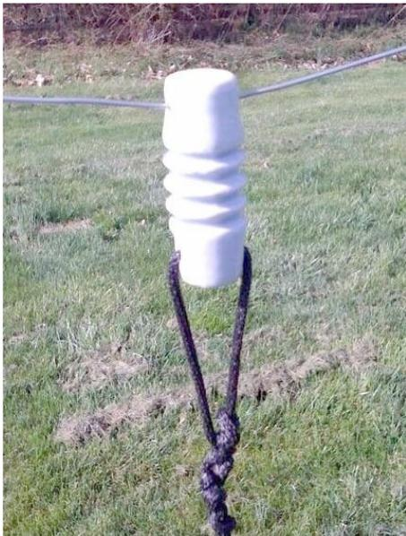
**Fig 1: A corner insulator, shown hanging down loose for clarity.**
