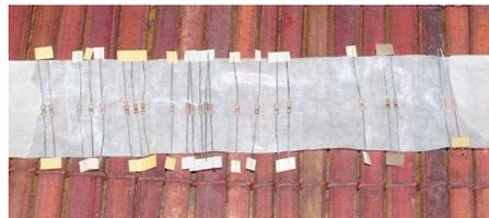
Photo 2. Resistors arranged on wide masking tape for easy access
