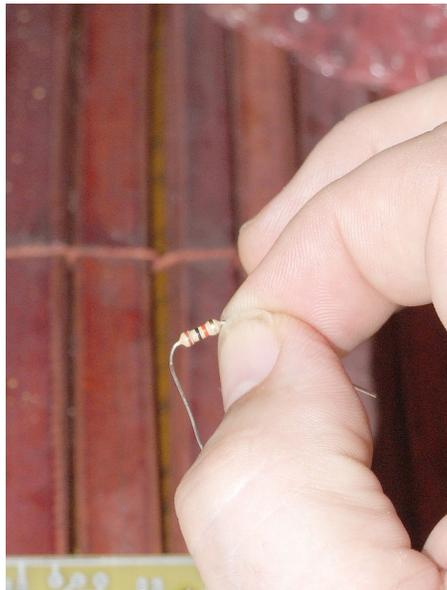
**Photo 5. Using thumbnail as a fulcrum for shaping leads on resistors and inductors**
