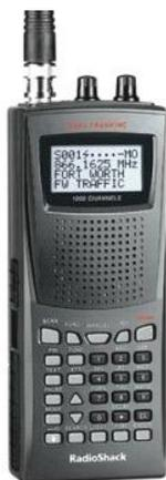
There might also be an easier way to achieve your goal of scanning individual talkgroups. The PRO-94 has the ability to scan specific talkgroup IDs held in lists in the scanner. Each of the 20 channel banks in the scanner can be used to track trunked systems. When a bank is used in this way, the scanner sets up five lists that can contain as many as ten talkgroup IDs. You could, for instance, set up one list for
