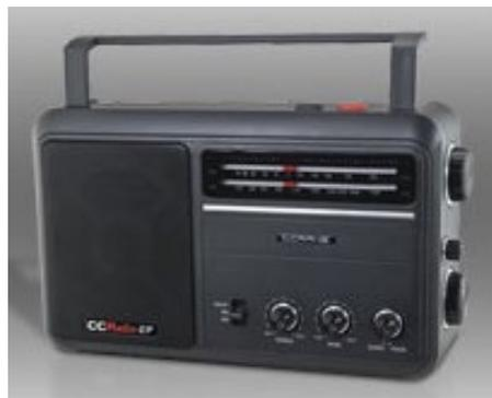
The radio has decent sound, good AM selectivity, wide/narrow FM selectivity, and external antenna connectors. It has the traditional, analog, slide-rule tuning dial which may be backlit for night viewing.
