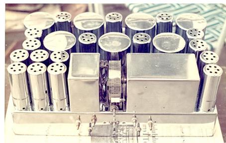
*The receiver chassis from the author's All-wave-23 when it was removed from the cabinet for cleaning in the mid-1970s.*
