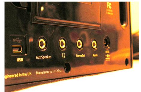
While most users will have some sort of WiFi option in their homes, it seemed odd that there was no Ethernet port on the Evoke Flow. This seems to be standard on most U.S.-made WiFi radios. The mini-USB option can still provide this functionality, but it requires a USB ethernet adapter, which few users are likely to possess. It seems to me it would have been easier to put an Ethernet port on the unit instead. This isn't a deal breaker, unless of course you prefer a hard-wired connection.
