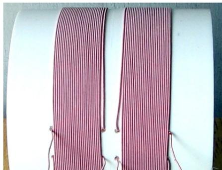
After winding, you will want to tension the wire. I found a procedure by which you can get a tight coil: After winding the coil, place it horizontally in your freezer for several minutes. The wires will get very loose because the styrene form shrinks. Take up the wire slack in the ends.
