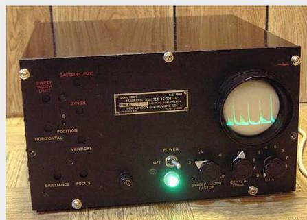
**Classic band scope:** This US Army Signal Corps BC-1031 panoramic adapter was used by Allied forces during World War II and later. An early spectrum analyzer, this BC-1031, built by New London Instrument Company, displays signals up to 100
