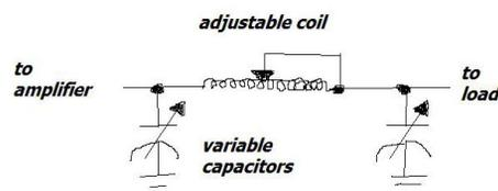
As a Novice in the early Seventies, I had an old Johnson Viking Ranger transmitter that had this pi network between the final amplifier and the antenna connector. I remember matching some really non-resonant antennas with this rig. We older hams used to say that the Ranger could match "a bobby pin on 80 meters, and a coat hanger on 160."
