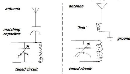
a wide range of impedance they could match. Transmitters, in particular, could match a wide range of loads, thanks to the discovery of the *pi network*. This circuit allowed the final amplifier of the transmitter to match to some really crazy loads. Thus, in a sense, the transmitter had its own
