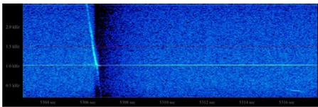
Meteor detection by radio was discovered around 1929-1930 by engineers while studying the effects on radio waves in the ionosphere (McKinley, 1961). They noticed short-lived enhanced signals on their recordings. Eventually, meteor radars were developed utilizing VHF (Very High Frequencies) to bounce signals off of the meteor trails. It enabled astronomers to detect the path, velocity, and duration of meteors. However, this technique is expensive and mostly out of the range of amateurs.
