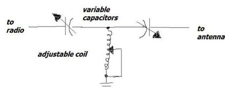
We could get ensnarled here in an arcane discussion of how this circuit works on a technical level, but that seems counterproductive. So here's a simplified way of looking at it: just think of the tuner as an adjustable transformer.
