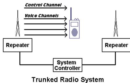
In a trunked system, things are much different. Any department is able to use any of the voice channels in the system. A conversation may jump from one frequency to another as different users take their turn talking. CTCSS tones are usually not used, but a control channel shared by all radios provides a means of coordinating what conversations take place on which voice channels.
