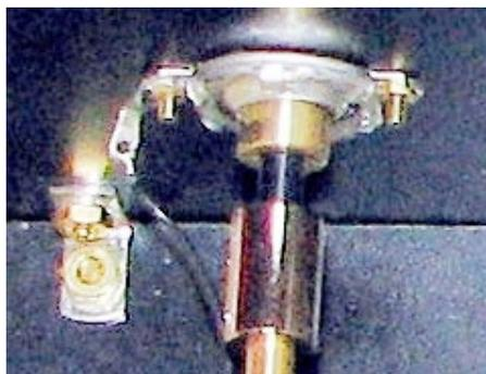
is done by attaching the three 1-1/4 inch long plastic standoffs to the bottom of each capacitor. A metal center point can be temporarily attached to the capacitor shaft with a shaft coupler. The point will accurately locate the height.
