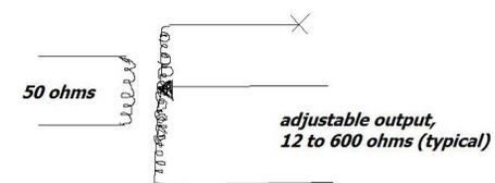
The only real restriction to all of this occurs if coaxial cable is used to run from the tuner to the antenna. Keep in mind that coax will not tolerate much of a mismatch (say 3 to 1 SWR or more) and the tuner cannot redeem this limitation. In other words, be aware that the tuner will be able to match a wide range of *random* (non-coax-fed) loads, but will only have a limited *useful* range of adjustment when feeding coaxial cable.
