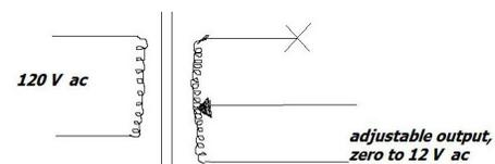
The antenna tuner can be visualized in exactly the same way. One side is connected to the radio's 50 ohm antenna circuit. The other side can be adjusted to a wide range of impedances, typically 12 to 600 ohms, allowing us to match a great many non-resonant antennas to the radio. (See Figure 5.)
