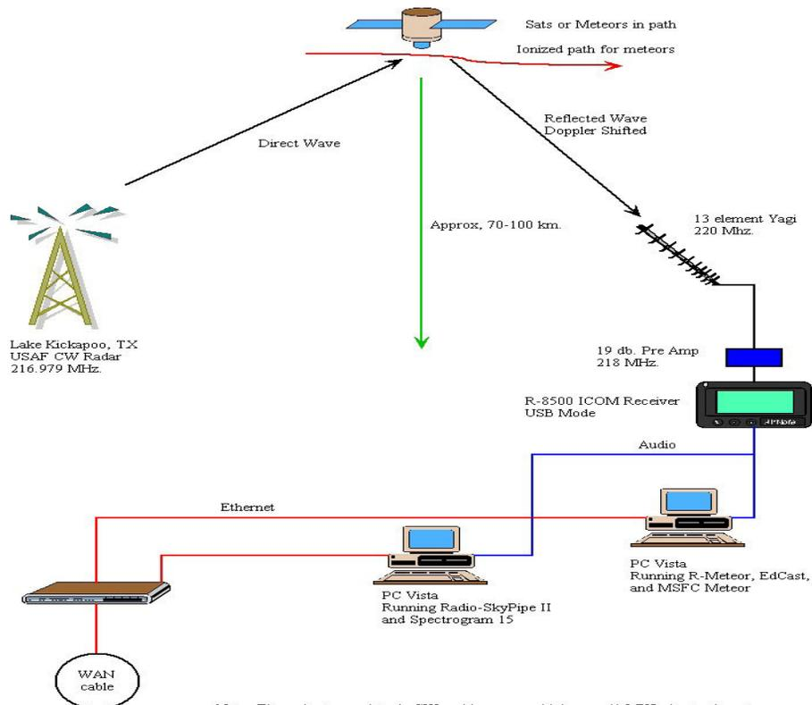
Note. The radar transmitter is CW and has a very high e.r.p (1 MW) due to the antennas. Usually meteors are not reflected well at this frequency but we overcome a lot of limitations due to the power. Also, NAVSPASUR uses a very narrow beam and Roswell is very close to the line that spreads across the US. Stan Nelson.
