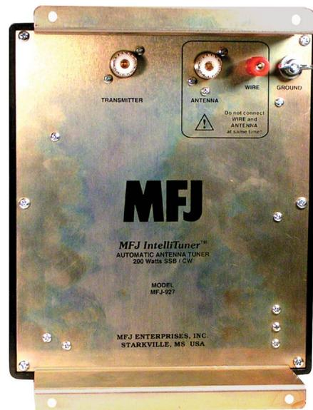
A typical remote automatic tuner. (Courtesy MFJ Enterprises)
