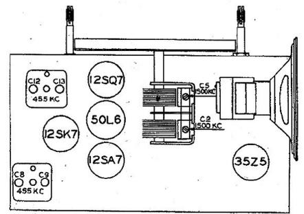
Fig. 3. Majestic chassis layout diagram shows location of all adjustment trimmers.
