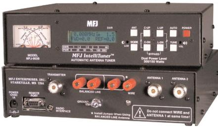
Front and back views of MFJ's dual-power automatic tuner. Courtesy MFJ Enterprises)
